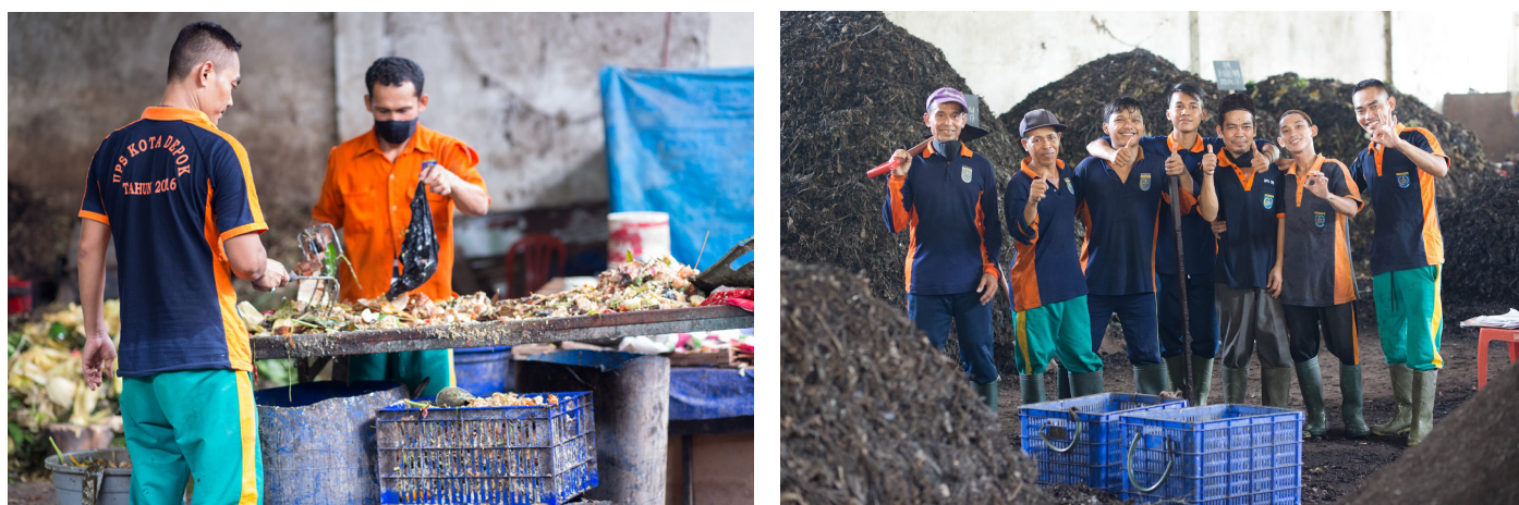
Figure 14: UPS (Composting Centre) in Depok. Organic Scraps Being Sorted to Remove Any Minor Plastic Pieces Wrongly Segregated, then Composted.
